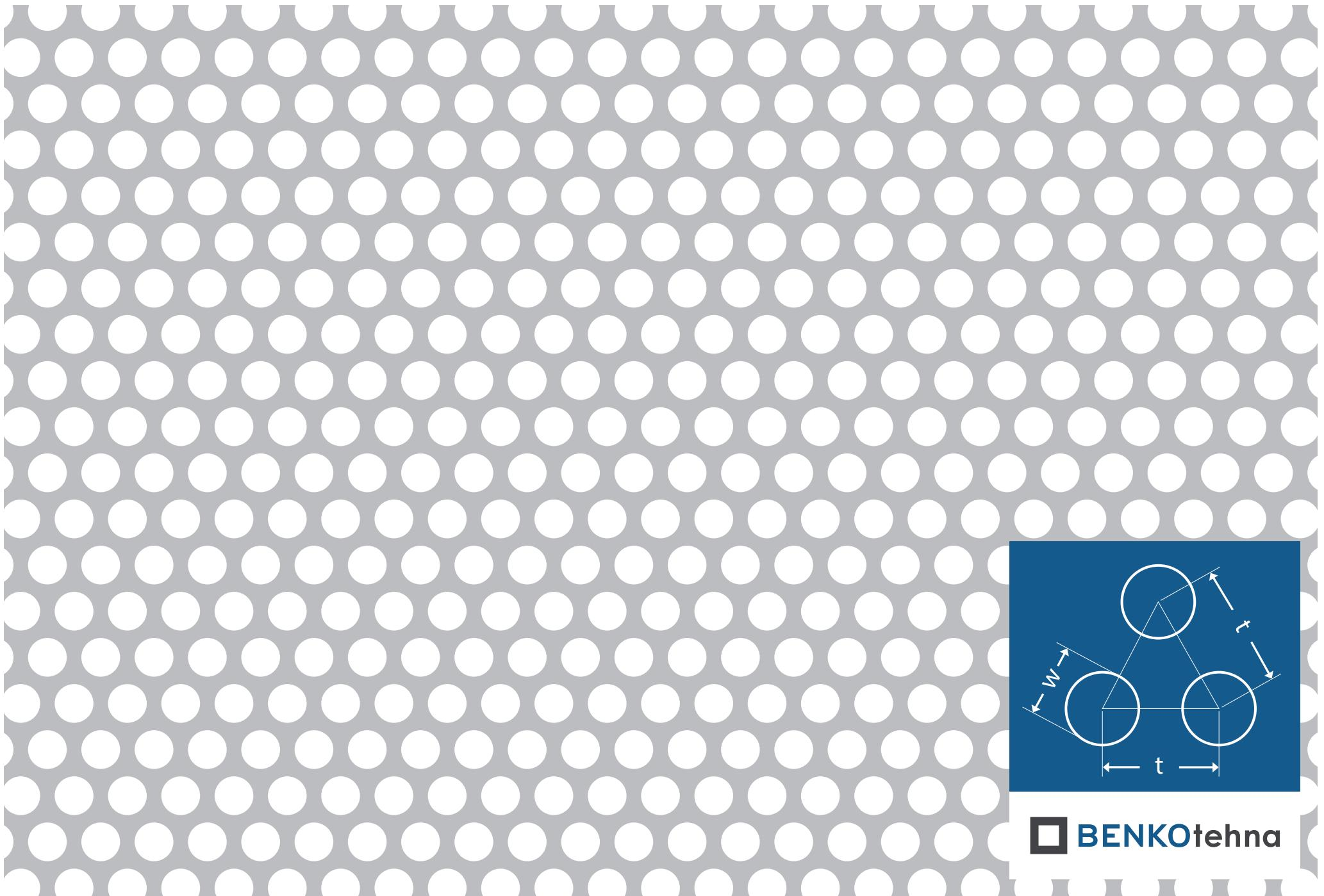
Okrugla s pomakom Op 8-11:  $w = 8,0 \text{ mm}$  |  $t = 11,0 \text{ mm}$  | otvorenost = 47,97%
