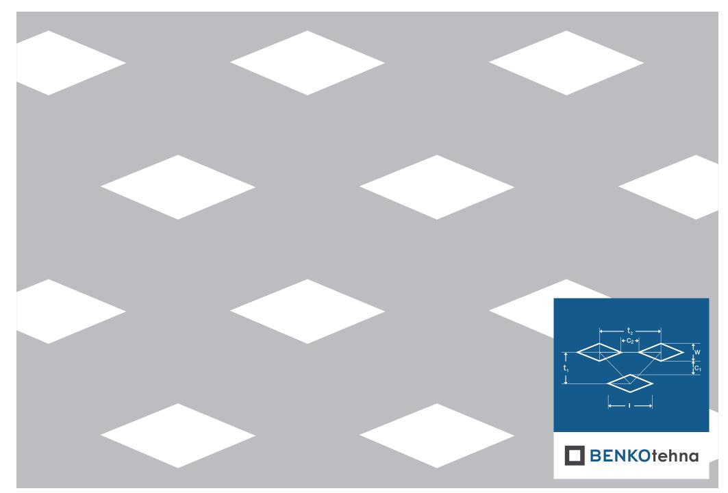
**CL** - **Romb s pomakom:**  $\mathbf{w} = 25,0 \text{ mm} | \mathbf{c_1} = 23,0 \text{ mm} | \mathbf{c_2} = 40,0 \text{ mm} | \mathbf{t_1} = 48,0 \text{ mm} | \mathbf{t_2} = 100,0 \text{ mm} | \mathbf{l} = 60,0 \text{ mm} | \mathbf{otvorenost} = 15,44\%$
