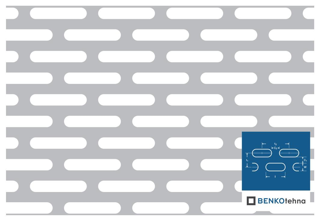
**Uzdužna s pomakom Up 10×50 - 19×60:** w = 10,0 mm |  $c_1$  = 9,0 mm |  $c_2$  = 10,0 mm |  $t_1$  = 19,0 mm |  $t_2$  = 60,0 mm |  $t_2$  = 60,0 mm | otvorenost = 41,97%
