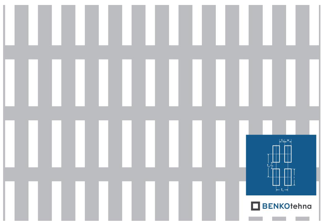
**Uzdužna redna Ur 8×40-20×52:**  $\mathbf{w} = 8.0 \text{ mm} \mid \mathbf{c_1} = 12.0 \text{ mm} \mid \mathbf{c_2} = 12.0 \text{ mm} \mid \mathbf{t_1} = 20.0 \text{ mm} \mid \mathbf{t_2} = 52.0 \text{ mm} \mid \mathbf{l} = 40.0 \text{ mm} \mid \mathbf{otvorenost} = 30,77\%$
